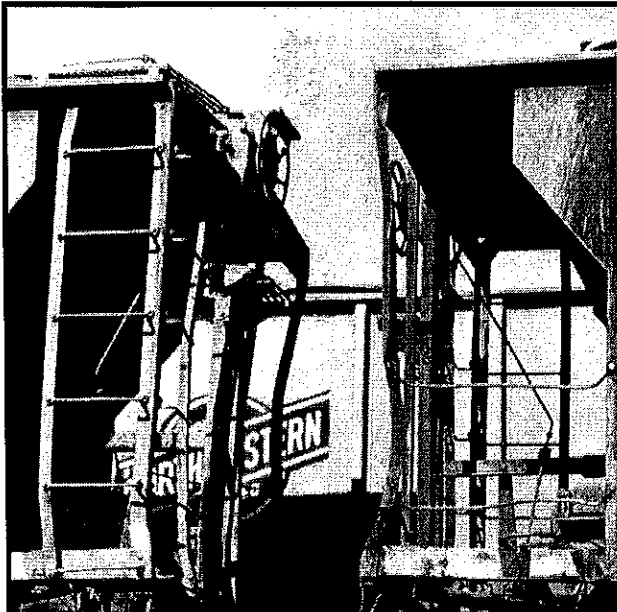
THIS PHOTO SHOWS THE "B" ENDS OF TWO PS-2 COVERED HOPPER CARS BUILT IN 1955. THE RETAINER PIPE, VISIBLY SILOUETTED HERE, ANGLES UPWARD FROM THE RIGHT SIDE OF THE CONTROL VALVE ON THE CENTER SILL TO A POSITION BETWEEN THE END LADDER AND HAND BRAKE.
