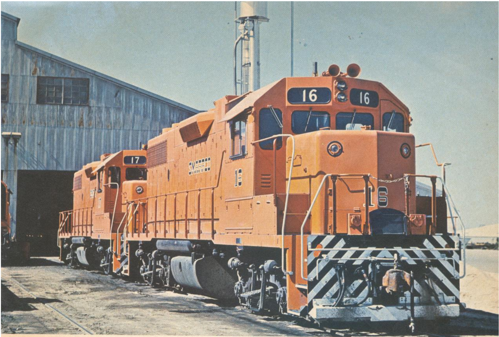
San Manuel Arizona has two GP38s seen here at the engine terminal. They handle switching chores as well as their regular road runs. David Lustig photo.
