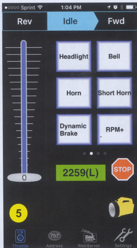
Above: The throttle window contains a sliding throttle; controls for basic CVs such as the headlight, bell, and horn; and an emergency stop button. The flashlight is the headlight. The assigned locomotive is shown in the green box. Forward, idle, and reverse are all shown at the top of the window.
